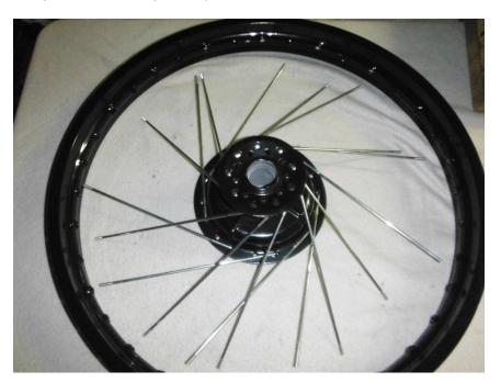
Now fit the outer spokes on the small hub side and fit them to the rim. These should also orientate clockwise. The spokes are approx. 245mm and have a 45 degree bend. See pic above.
