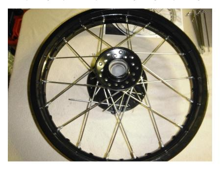
You can now fit the inside spokes on the large hub that you first fitted. They should just swing down into position and into the correct dimple. See pic above and below....
