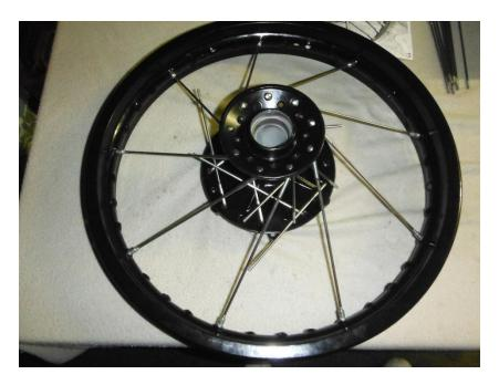
Now, insert the inner spokes on the small side of the hub and swing them around in a anti-clockwise direction as per the pic below and fit them to the corresponding dimple. Notice they fit underneath the other set of spokes you just fitted to the rim. Count the dimples as per my pic and look for the corresponding dimples. Take your time to get it right as you can go a bit wrong here.
