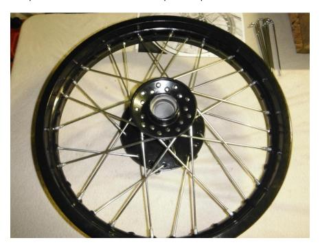
Finally, you can fit the last 90 degree bend spokes on the outside of the large side. Drop them down through the top, lean them anti clockwise and fit them to the rim using the last remaining 8 nipples as per the pic below. Use a Philips screw driver to nip all the spokes up and this wheel is ready for truing. Let's move onto the front rim....
